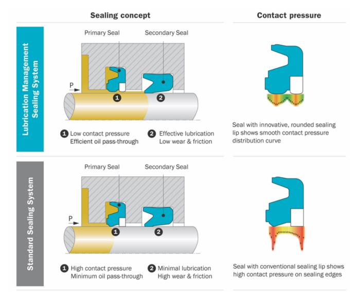
Lubrication management reduces heat and minimizes wear between primary and secondary seals.
