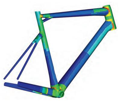
Simulating the general stress distribution on parts and the way composite layers are affected by it go hand in hand. These examples show how the process works in ANSYS simulation software. Images courtesy of ANSYS.
