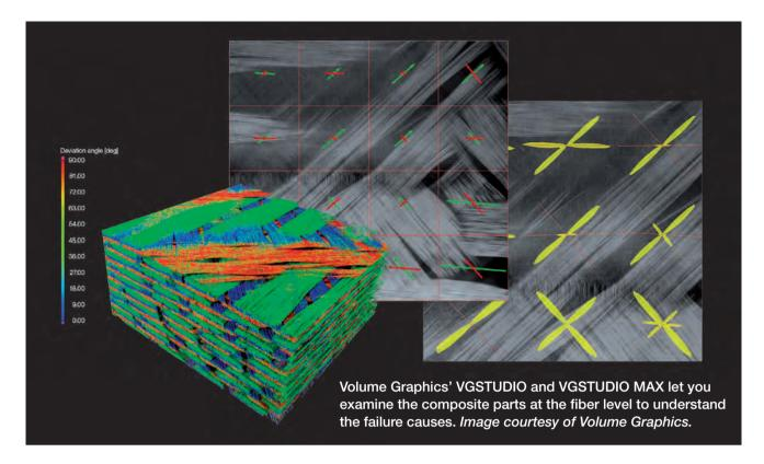
affects how they perform and behave, so it's critical to be able to simulate the design process," remarks Assaker. At the stage where reinforcing materials, such as glass fibers, are added to the base material, called the Matrix, the orientation of the fibers determines the strength of the final product when pulled or stretched from a certain direction.
