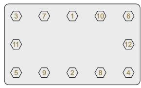
Make sure to install the gasket with sufficient surface pressure.
