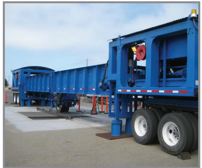
HVS testing on the deck joint
